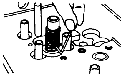
Figure 4-7. Bridge Guide Removal Tool, Installation.
